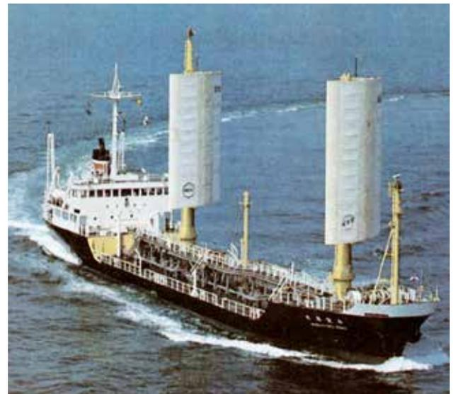
Wind-assisted propulsion using wingsails in the 1980s.
