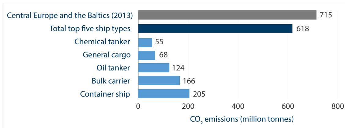
Figure 4: CO<sub>2</sub> emissions by ship type, showing a comparison with land-based emissions.
