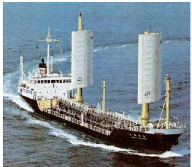
Wind-assisted propulsion using wingsails in the 1980s.
