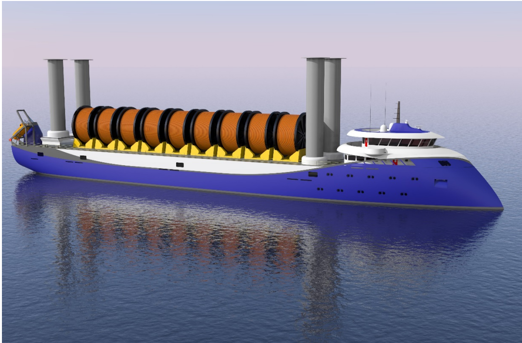
Figure 6.1: 3D-render of the Flettner Freighter Concept
