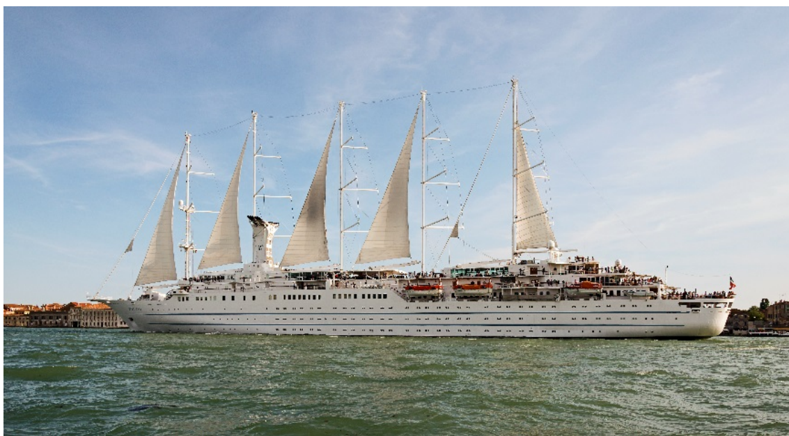
Fig. 2.3: The „Wind surf“ has a rather traditional rig which is completely computerized and does not require extra crew. (Photo: Didier Descouens, CC BY-SA 4.0)
