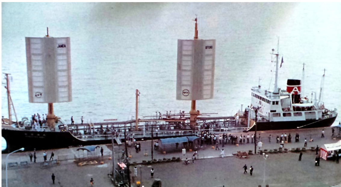
Fig. 2.2: The “Shin Aitoku Maru”, a successful hybrid driven ship from the 1980s. (Photo: Mkmillenium. CC BY-SA 3.0)
